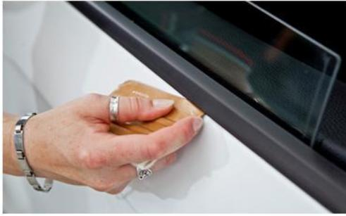
**Important Notice** Partial wrinkling of the film may occur at window trim gaskets because of possible mechanical movements of the gasket resulting in stress on the film.
