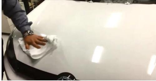
Note: Do not use isopropyl alcohol as this can affect the adhesion of the film. Other solvents than 3M™ Surface Preparation System may affect the adhering properties of the film, too.
