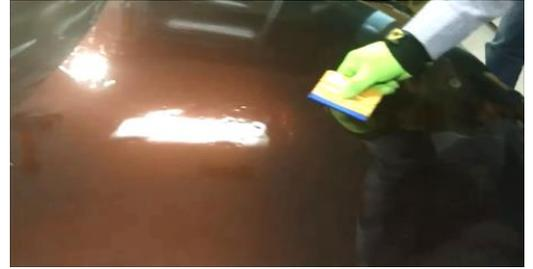
Apply the film with your finger in concave parts where necessary and continue squeegeeing.
