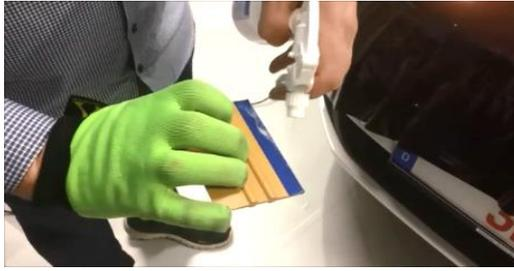
Apply the film lengthwise from the center outwards with overlapping strokes and ensure that the squeegee is in constant contact with the film. 3M Controltac technology ensures that the film is flexible on the surface and adheres only when pressure is applied, whilst 3M Comply technology allows air to be easily removed without causing bubbles.
