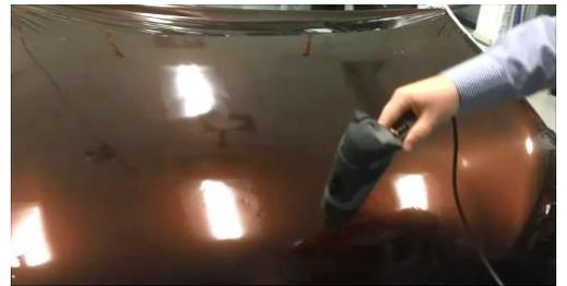
By heating the film and letting it cool down, wrinkles disappear and the film will conform to the surface so that squeegeeing will be possible without repositioning of the film.
