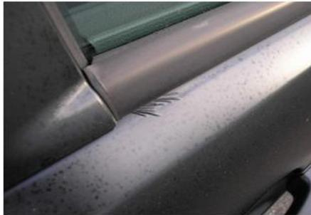
**Important Notice** The wrapped vehicle should remain in the shop floor for at least 24 hours to allow the adhesive to build up adhesion on the car paint. Car wash should not be done before 7 days after wrapping.
