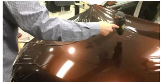
The film surface should reach a temperature of +30°C to +40°C.
