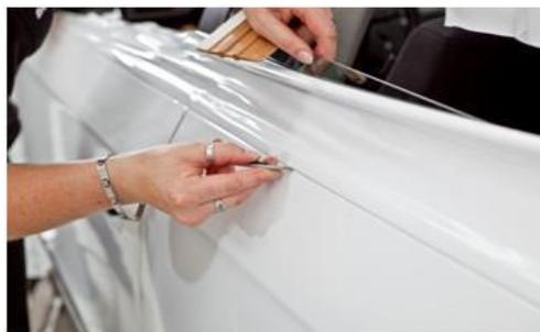
Cut the film at an overlap of approx. 2 mm on the gasket and apply the film with the squeegee underneath the gasket. For cutting the use of Knifeless Tape is recommended.
