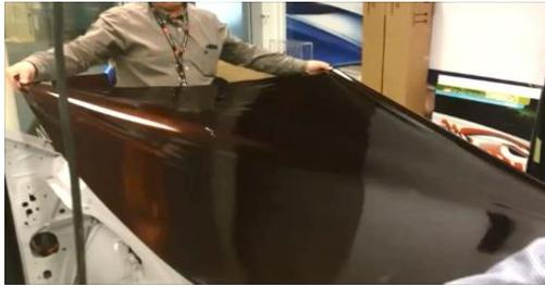
Span the film with low tension on the substrate to remove larger wrinkles but do not stretch the film at the edges.
