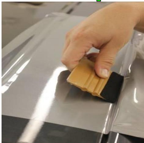
It is very important NOT to squeegee the film directly after heating. Let the film cool down for a few seconds after heating, then firmly squeegee without stretching the film. Stretching at the edges might cause shrinkage of the film and color fading.
